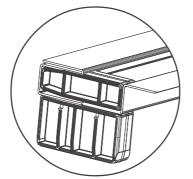
Remove the remaining head joiner out of the strike jamb into the end of the head (as shown) to receive the strike jamb.
