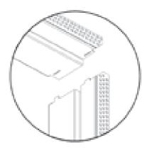
Locate fixing tabs to header.
