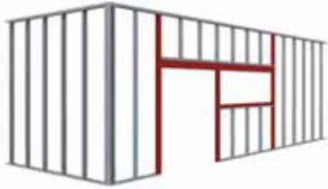
Openings in external walls
