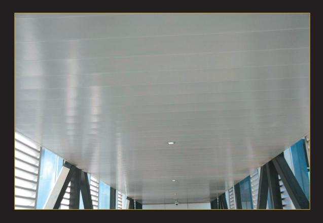
HARMONI 180 is an elegant ceiling system that can be used in a broad range of applications. The 180mm wide monolithic panel provides a wider concealed fix system that gives greater focus to the ceiling plane whilst retaining plenum access. HARMONI 180 is equally effective in small and large spaces and has a non-woven bonded acoustic backing which delivers premium acoustic performance.
