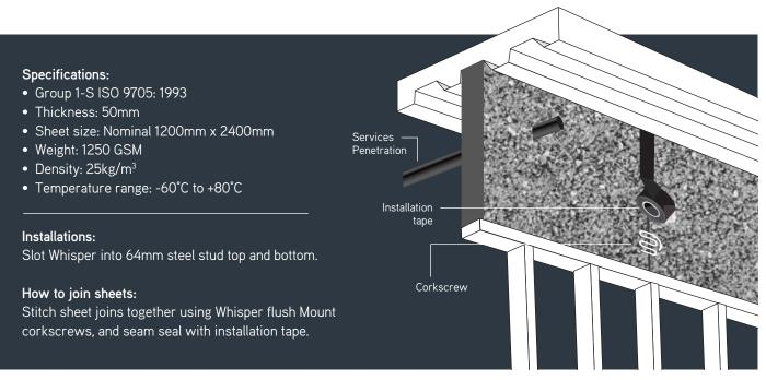
Whisper should not be used near heat sources exceeding this temperature range. Where the ceiling plenum is used as an active return by the HVAC system, ensure airflow is not reduced by consulting a Mechanical Services Engineer.
