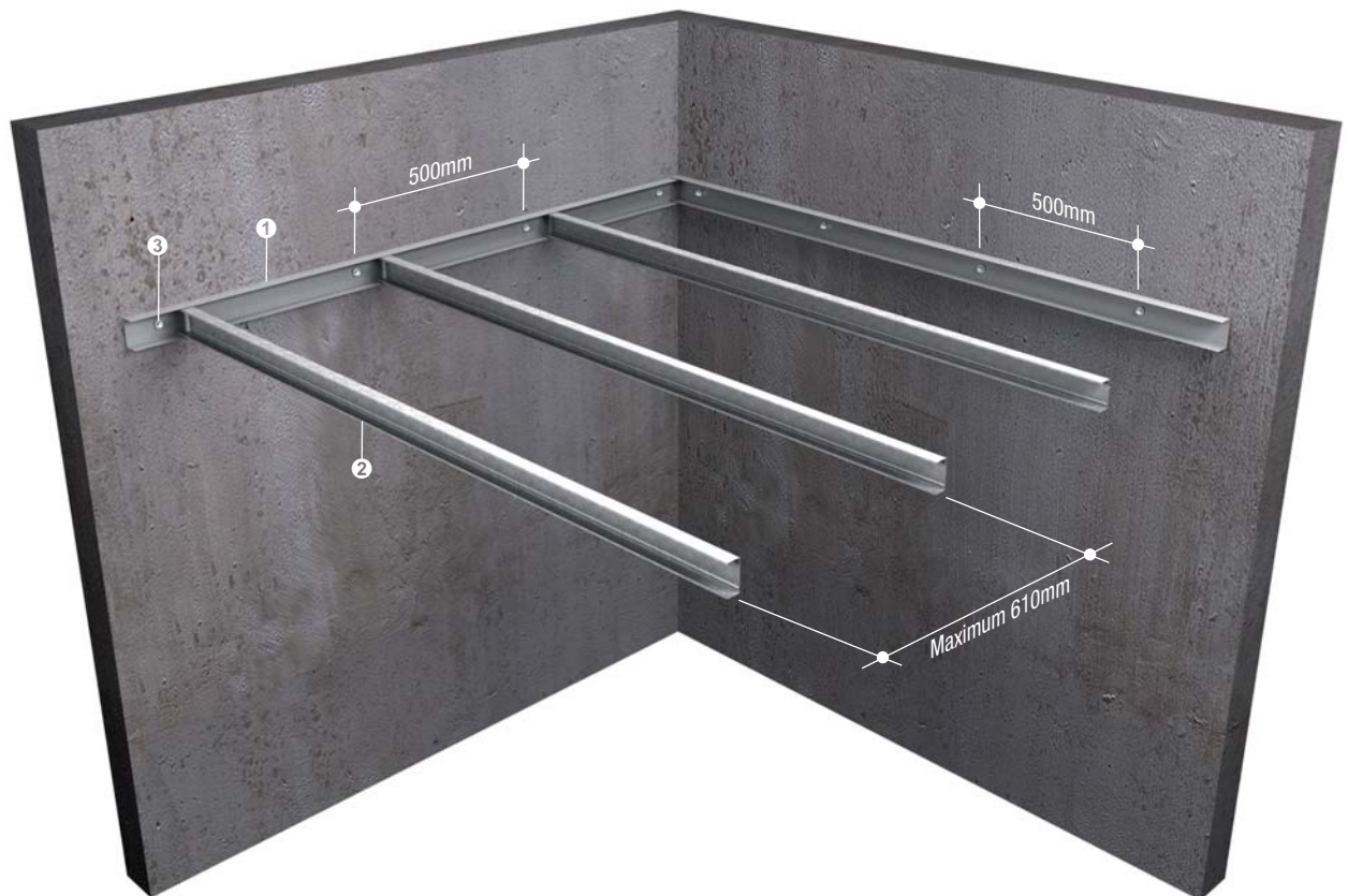
Fixing of primary and secondary profiles
