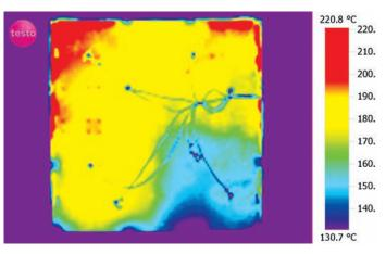
The panel was heated up to a temperature of 1000°C (1832°F) for 2 hours until steady state was achieved. Thermocouples were placed on the cold face (casing) of the 4 zones to follow the temperature evolution in real time.
