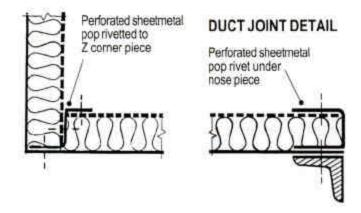
Ductliner/Siliner should be fitted and adhered to the internal surface as described before (see Velocities up to 12.5m/sec).
