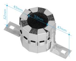
A Fire Resistance Level (FRL) of up to -/240/240 in accordance with AS1503.4:2014, AS4072.1:2005 and BS476: Part 20: 1987 can be achieved on selected combinations of pipe and substrate. Approvals available for PEX, uPVC Conduits, PEX/AI/PE and many other pipes types. Consult the <u>Promat Fire Collar Selector App</u> to ensure your specific combination is approved.
