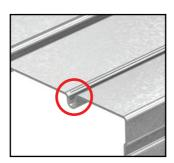
The 120mm top hat is supplied with two expansion zones in the fixing face, to allow limited expansion and contraction to occur where two lining boards join.
