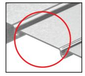
For a weather-tight seal in express jointed facade systems, the central portion of the fixing face is recessed to allow for a self-adhesive foam backing strip.
