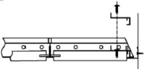
A minimum of two Tegular Border Clips (Item BP6044) to be screw fixed to each cut panel.
