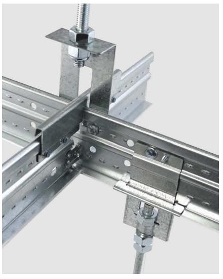
Integrated hanging clips allow connection to M10 threaded rod for flexible and reconfigurable overhead cable tray and electrical distribution without a separate strut channel system.
