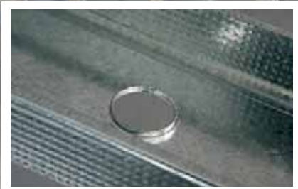
Service Holes Bell-mouthed service holes at 500mm centres – do not require grommets for cabling. Knurled face for screw point location.
