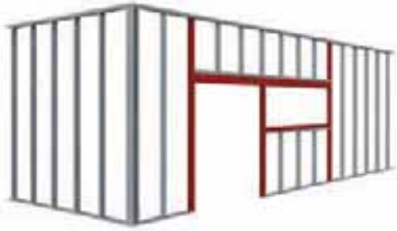
Openings in external walls
