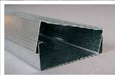
Boxed Studs Studco .50, .55 and .75BMT steel studs can be easily boxed together providing extra strength at door openings or where greater loads are required.
