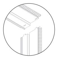
Locate fixing tabs to header.
