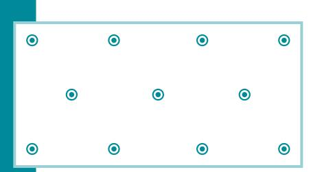
Suggested layout of fasteners on a 1200 x 2400 sheet
