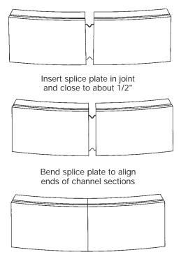
Close joint and tighten screws
