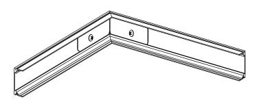
Splice plates are shipped flat. Hand bend as required for mitered intersections.
