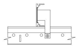
When used to align grid members that extend beyond the bottom of the trim, the clip is secured to the web of those grid members using a standard framing screw supplied by the installer. One clip is required at each grid/channel intersection.
