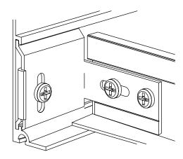
T-Bar Connection Clips are attached to the grid members using screws supplied by the installer. Framing screws (#6 x 7/16" or 1/2" lg.) are typical. Special conditions such as open cell installations may dictate the use of alternate methods of attachment.
