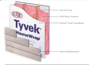
Tyvek® HomeWrap® is a fire retardant synthetic non-woven high density polyethylene (HDPE) homogenous sheet, manufactured using a spun-bond process. Specifically treated to provide high water resistance, high water vapour permeability (to assist in managing moisture in the wall cavity) and high air barrier technical properties.
