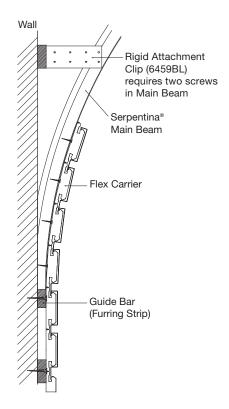
**4.5.1** METALWORKS F-Plank can be installed to create a curved transition from ceiling to wall by using (only for 100mm wide planks) faceting drywall grid main beams.
