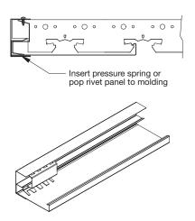
**3.16** Cut the panels to length to fit into the perimeter moulding at the sides, parallel to the carrier. Cut end will fit into the lower channel. Use pressure springs on ends as needed.
