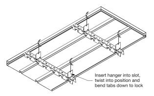
**3.8** Fasten the carrier to the moulding at the proper location, align the notch as indicated in Section 3.6 and fasten with a framing screw or pop rivet. Notch the carrier to fit into the wall moulding as needed.
