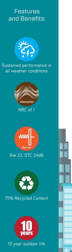
**WhisperFence™** 24dB is a unique combination of our patented Stratocell Whisper UV with a recycled barrier material to improve transmission loss. The light weight, easily managed, semi rigid panels are quick and simple to install vertically as hoardings on construction sites, acoustic fencing and noise barrier walls.
