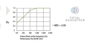
Wet-formed mineral fibre with durable acoustically transparent membrane
