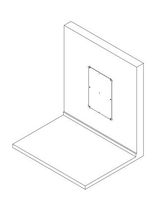
Attach stencil to wall using tape or staples etc.
