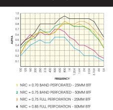
5 NRC = 0.45 UNPERFORATED - 25MM BTF6 NRC = 0.60 UNPERFORATED - 50MM BTF
