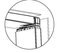
Locate head into joiner and make flush with jamb so the head joiner is not seen.
