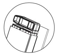
Head joiners as inserted in jamb.
