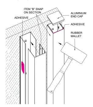
End caps can be supplied for all Snap On Baffle profiles and are friction fitted. When installing End Caps, apply a "thumb print sized" dab of construction adhesive to ensure suitable fitting.
