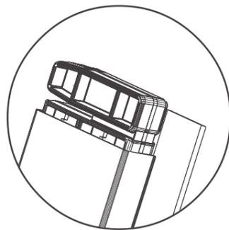
Head joiners as inserted in jamb.
