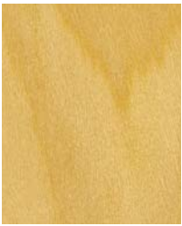
HP(L)(V) – Hoop Pine Rotary Cut
