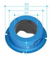
Note: The FWR 100 type suits 100mm, 80mm and 50mm uPVC pipe with a fitting.
