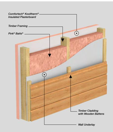
**Figure 1.** Comfortech® Kooltherm® Insulated Plasterboard lining on a traditional timber framed wall with R2.8 Pink® Batts®. Bracing components are not included in the figure.
