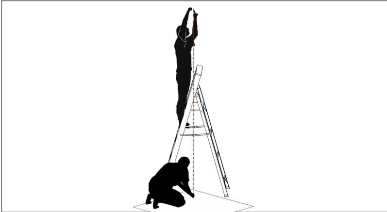
Lay supplied stencil on ground directly below ceiling surface you would like to install your Vista panel.
