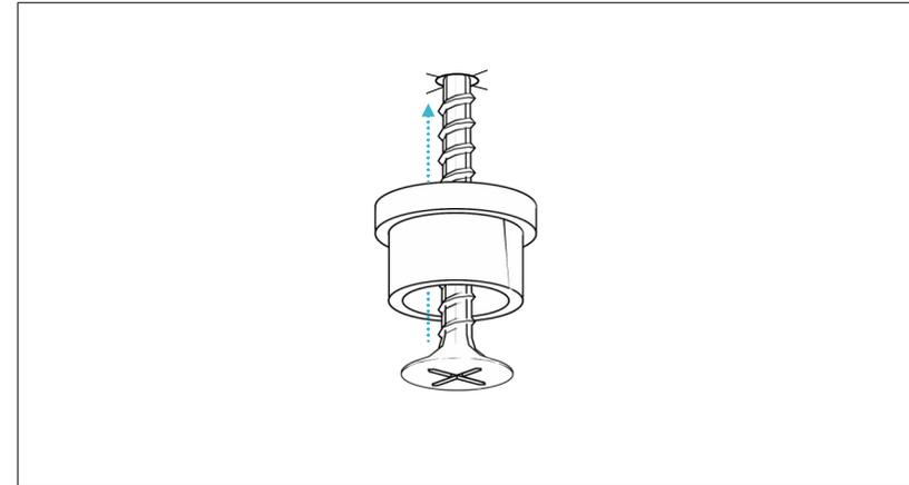
Insert supplied screws\* into adjustment 1 and screw into ceiling at marked spots.
