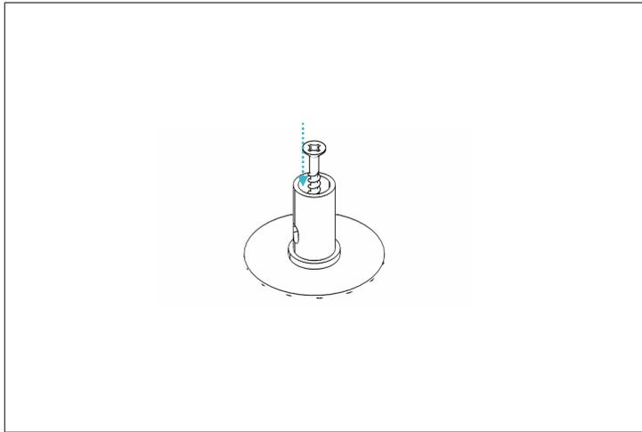
Screw adjustment 4 to base, rear of panel, until fixed tightly.
