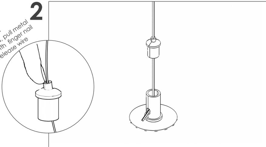
Thread wire a few inches through Adjustment 3. Insert wire through adjustment 4. Screw both adjustments till tight.
